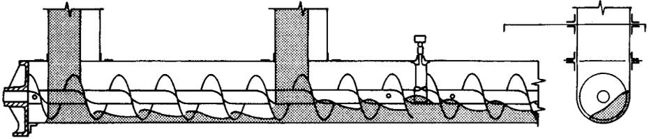
Fig. 38.1 Chute-fed screw conveyor.
