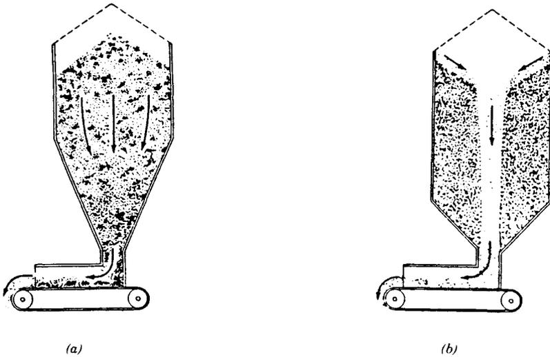
Fig. 38.7 Mass-flow (a) and funnel-flow (b) in storage bins.
