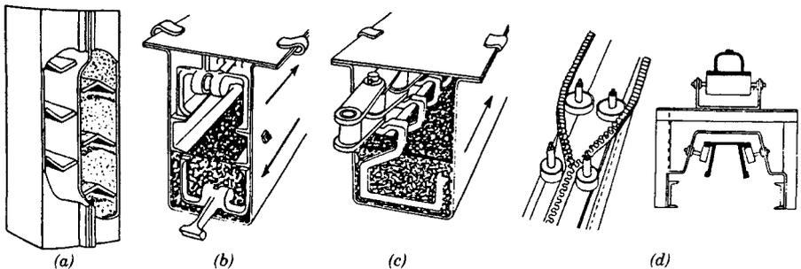
Fig. 38.5 Continuous-flow conveyor.
