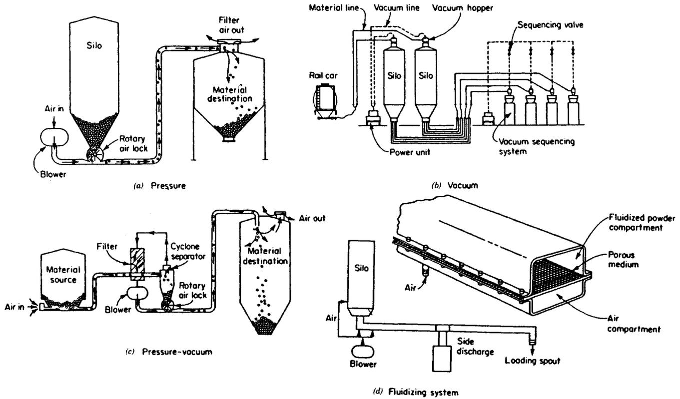
Fig. 38.6 Four types of pneumatic conveyor systems.
