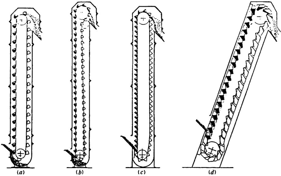
Fig. 38.3 Bucket elevators.
